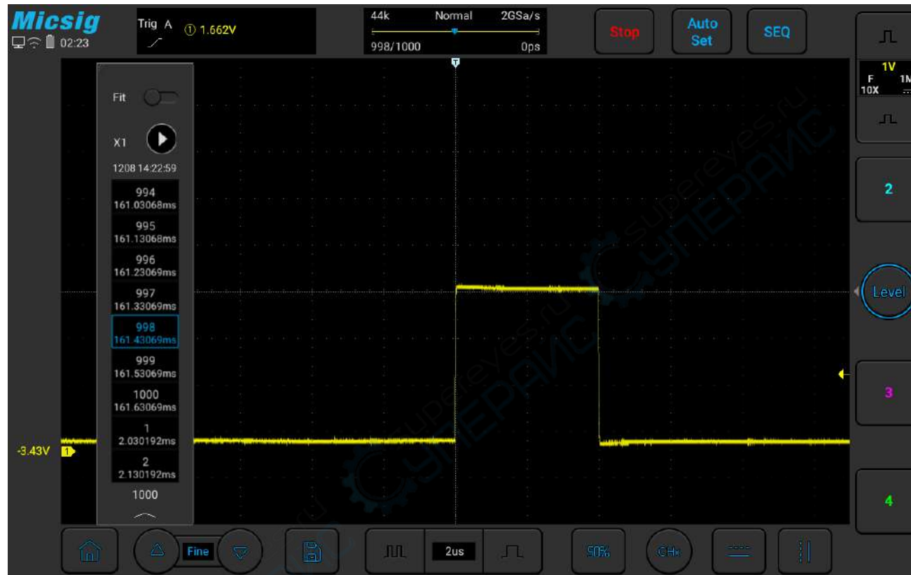
Figure 10-12 Single frame view of segmented storage
