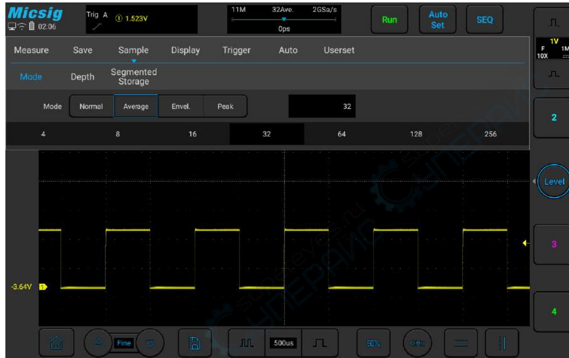
Figure 10-7 Waveform after choosing the average sampling mode, with average number 32
